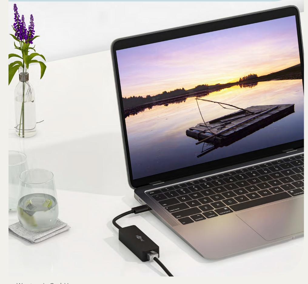
USB-C™ LAN adapter for a full-duplex network connection with 10/100/1000 Mbit/s via the USB-C™ socket of a computer
